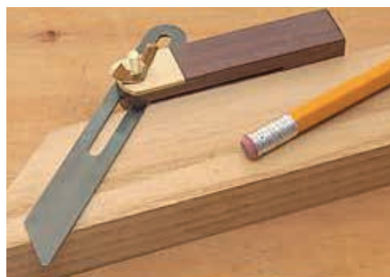
Transferring angle from bevel to the job
